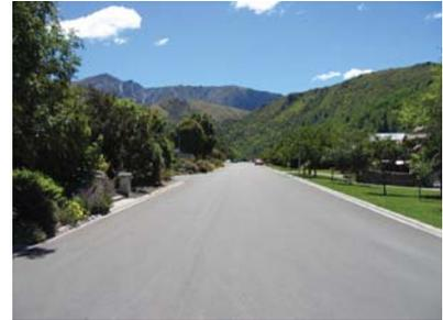
Try to avoid excessively wide carriageway with low profile kerb and channel.
