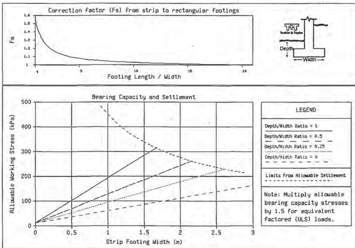
Figure 7.1 and 7.2 have been developed based on methods recommended by Peck Hanson and Thornburn (1974).
