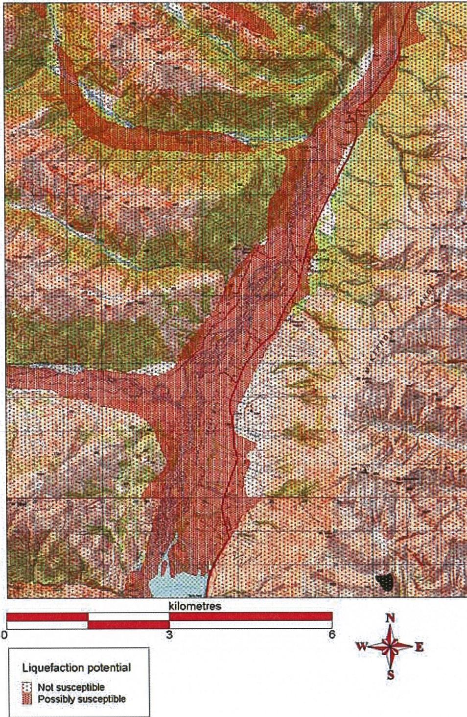
Figure 8: Land possibly susceptible to liquefaction induced by seismic shaking.
