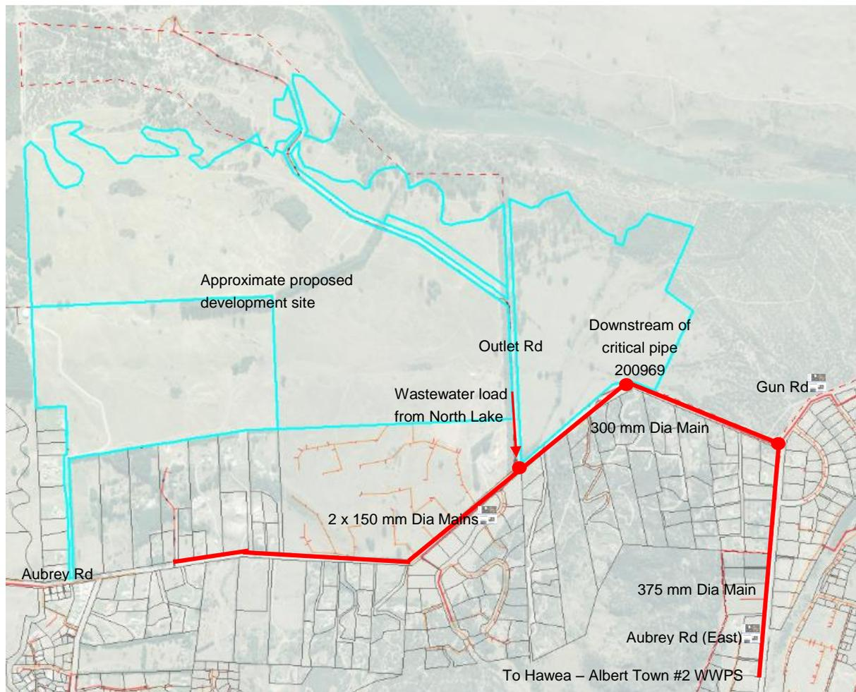
Figure 1- Wastewater schematic
