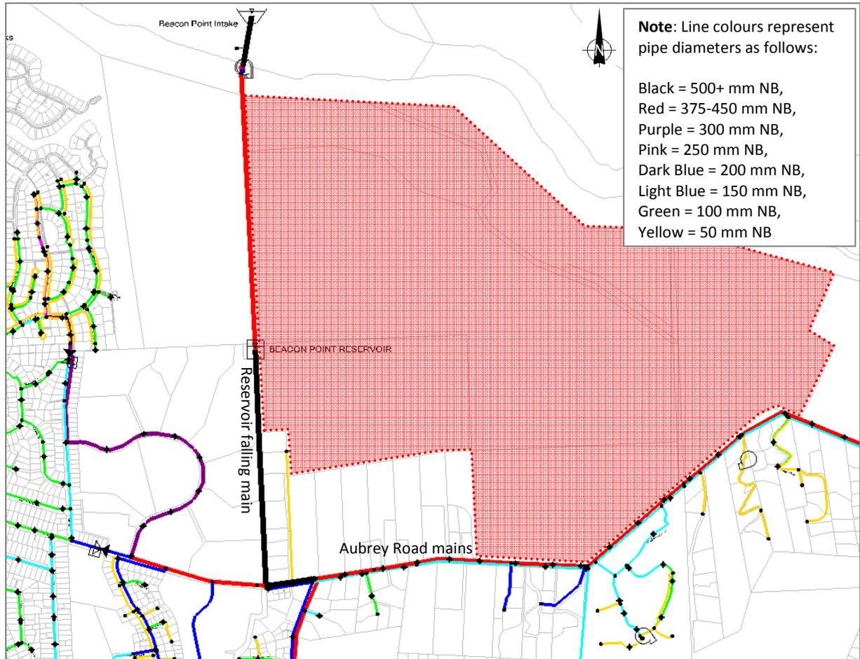
Figure 1 Wanaka water supply network near the proposed rezoning (site outlined/shaded in red)
