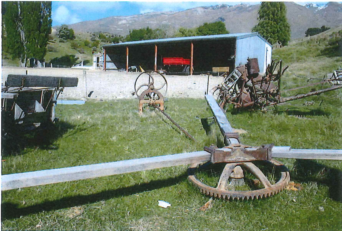
Figure 3 Reid and Gray's three-horse power whim, restored to its original configuration.
