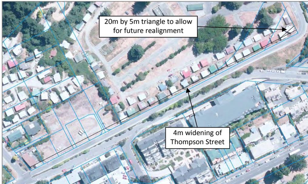
**Figure 7: Proposed roading designation for inclusion in the Plan Change to allow for future realignment**
