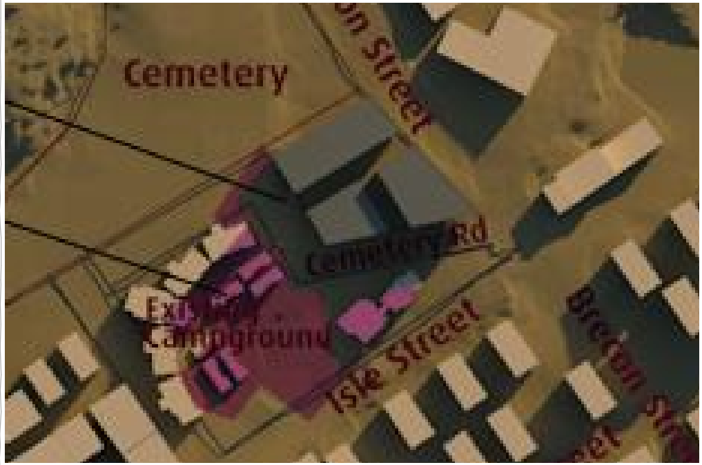
June 21, 2015, 10am: Sun Altitude = 11.6183° Sun Azimuth = 51.4595° Building Composition Comparison: Comparison between a 12m building and a 24m building on 34 Brecon Street using the BSPL building composition and the existing campground. The additional shadows from 24m building are shown in pink.
