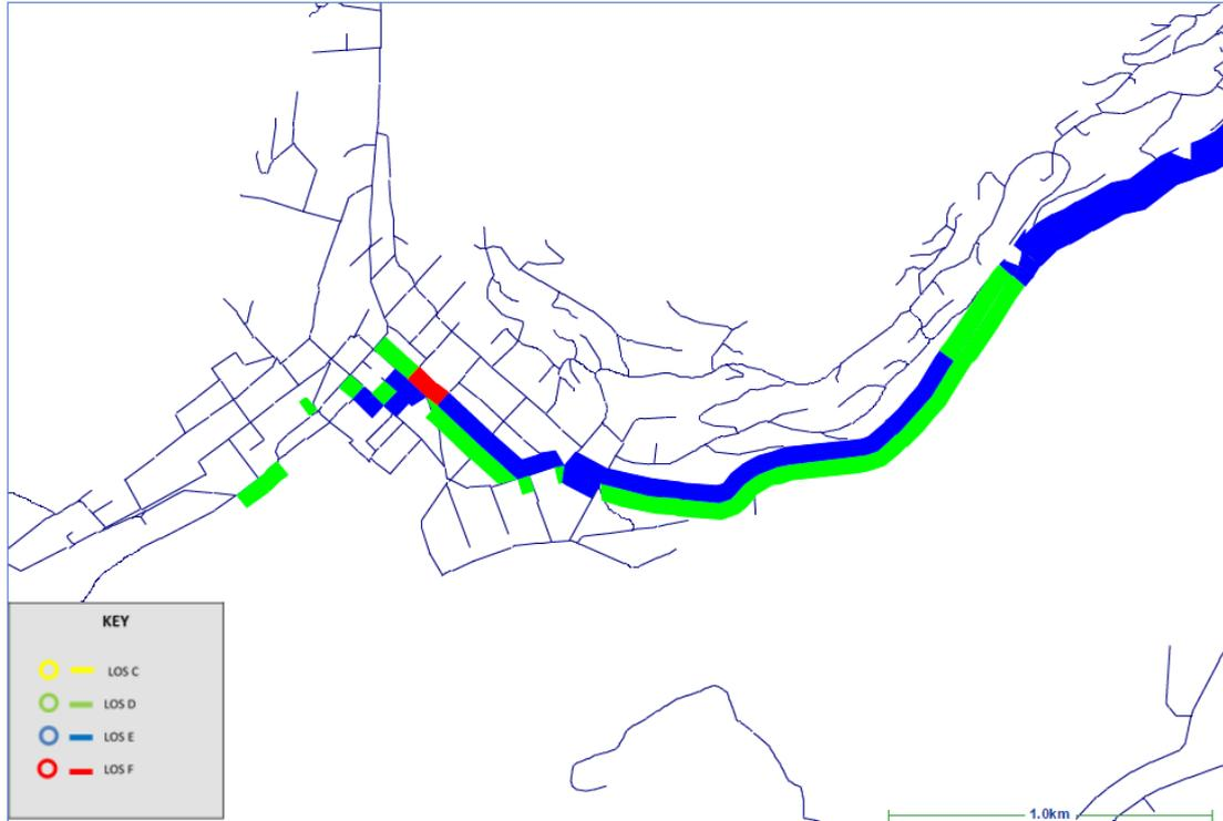
Figure 11: 2025 PM Peak Level of service – do minimum (no arterials)
