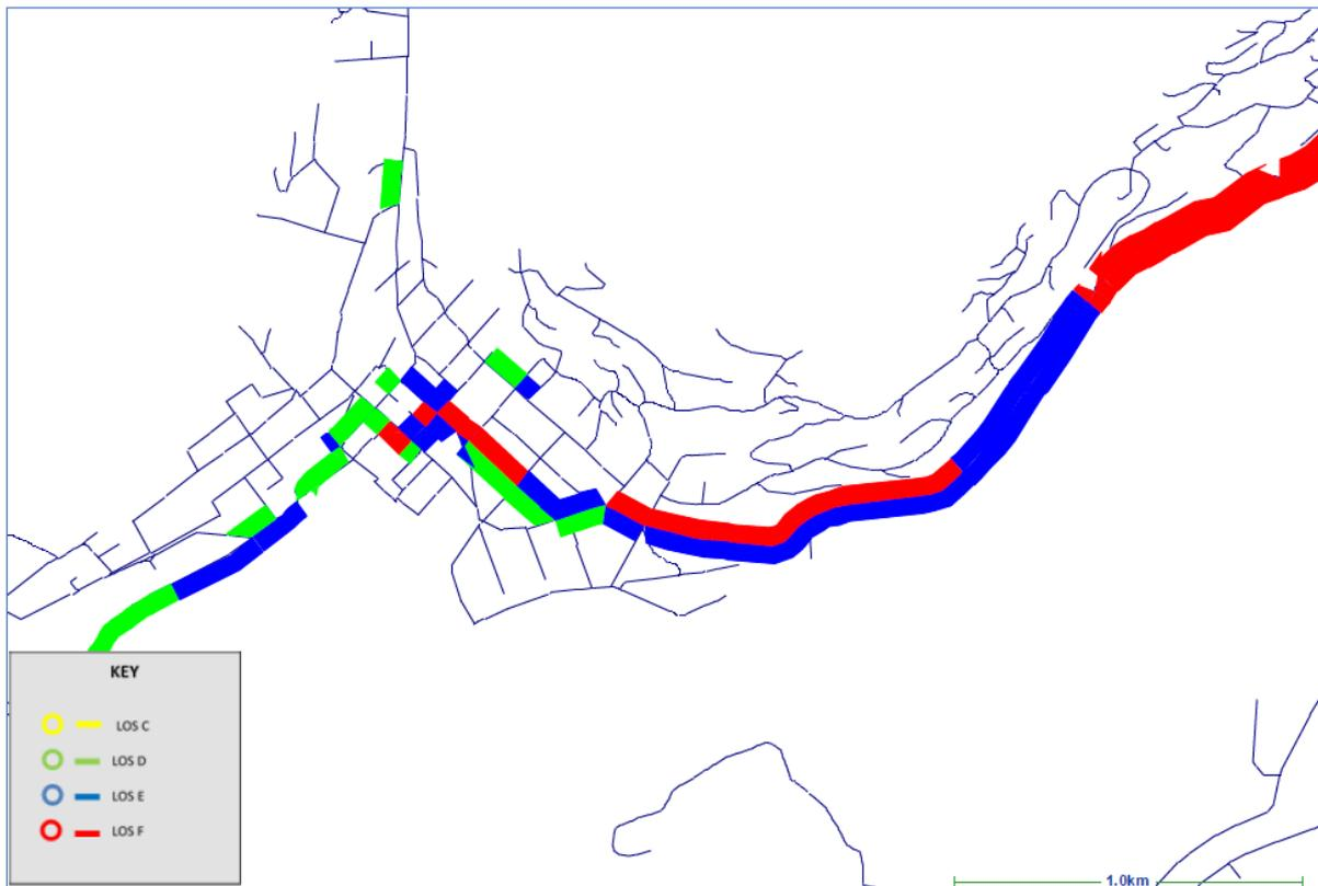
Figure 12: 2045 level of service plots under a do minimum scenario (no new arterials) - PM peak
