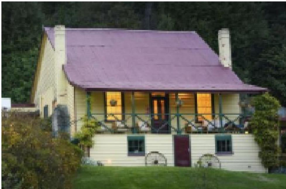
From my review of the photographs you provided the single level building structure comprises light weight timber framing for floors, walls and roof and there are two tall brick chimneys to each of the gable ends. Timber framed structures of this type are not typically earthquake prone but the two chimneys would be unless strengthened.
