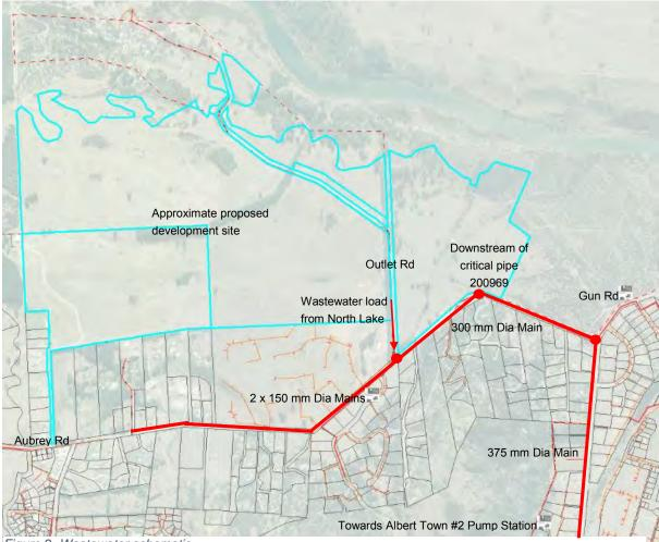
Figure 2- Wastewater schematic
