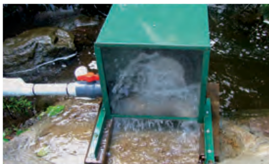
Figure 49. A micro-hydro turbine using a Pelton wheel Photo credit: Ecolnnovation
