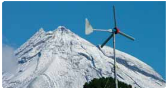
Pole-mounted, with guy wires, three-bladed horizontal-axis micro wind turbine. Photo: EcolInnovation
