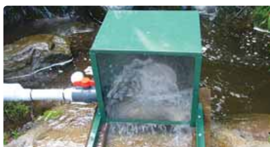
Close-up of a Pelton wheel impulse turbine. The water returns to the same catchment that it was diverted from. Photo: EcolInnovation
