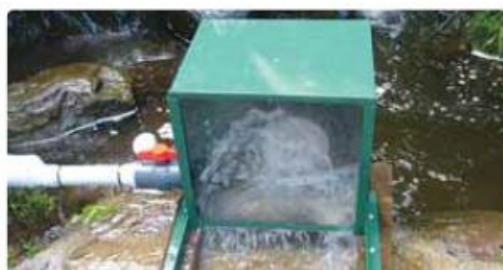
Close-up of a Pelton wheel impulse turbine. The water returns to the same catchment that it was diverted from. Photo: Ecolnnovation
