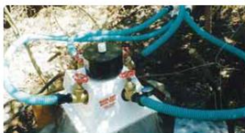
A Turgo impulse micro hydro turbine. Photo: Alternative Power NZ Ltd.
